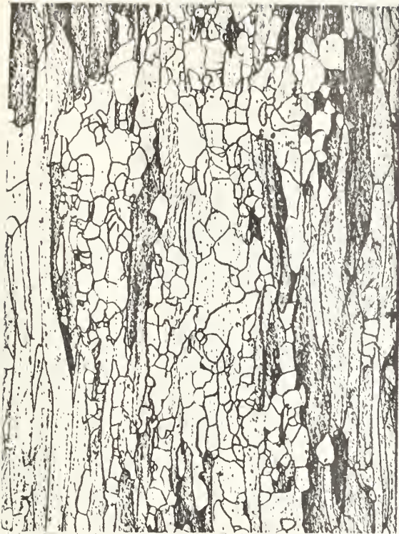
FIG.13 AT 597°C FOR 2 MINUTES (ROCKWELL 30T 52.6) -150 X- FIG.14 AT 540°C FOR 42 MINUTES (ROCKWELL 30T 51.9)
